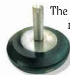
The RoughDeck was engineered to use a steel and neoprene sandwich design called SUREFOOT™. A steel cup sits on the floor and is bonded by a pliable neoprene cushion to a steel top plate with attached threaded stem. This pliable sandwich allows the stem and top plate some plasticity to move laterally and tilt independently of the bottom steel cup. This allows the foot to accommodate small deflections and uneven floors.
